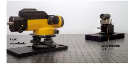
**Fig. 3** Photographic layout of measuring application of collimated VCSEL array performance (Source: Duma Optronics)
